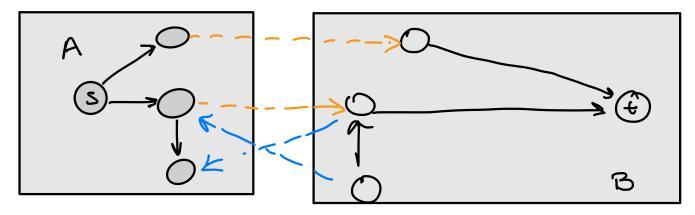
$$val(P) = \sum_{e \text{ out of } A} f(e) - \sum_{e \text{ into } A} f(e)$$
